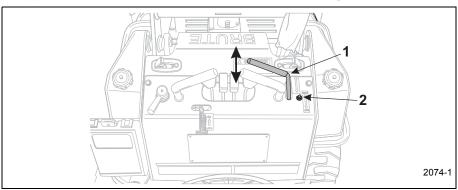
Figure 3-29 Auxiliary Control Lever
